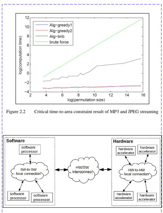
Figure 3.3 Communications among hardware and software tasks in a multi-core architecture (Cheng, 2018)
